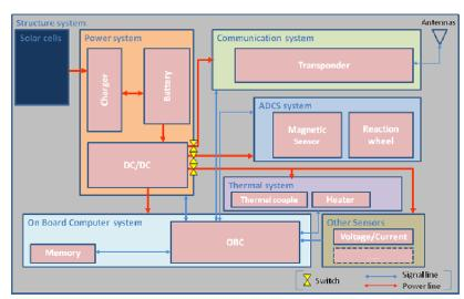
Figure 3: System function blocks
